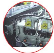
Bonding Mechanism & X-Y Axis Assemble 焊接装置 & X-Y轴传送装置
